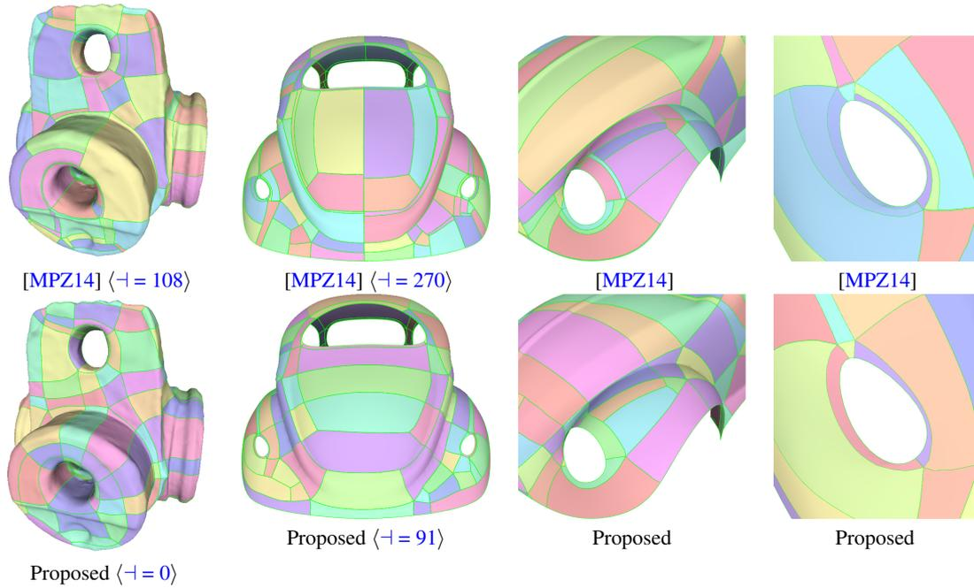
**Figure 16:** (Our method reduces the total number of  $t$ -junctions with respect to [MPZ14]. As a consequence, the zero loop generated by [MPZ14] (about the hole in the close-up) vanishes implicitly in our final layout (right).)
