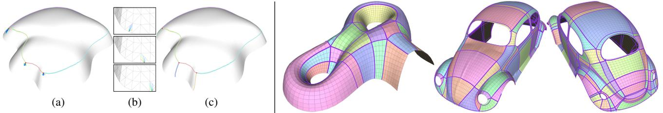
**Figure 8:** Left: some nodes may be unsolved because they need to be connected with the border (a); it is sufficient to propagate paths from the singularity until they reach the border (b) to complete the patch layout (c). Right: some examples of models with multiple complex borders.
