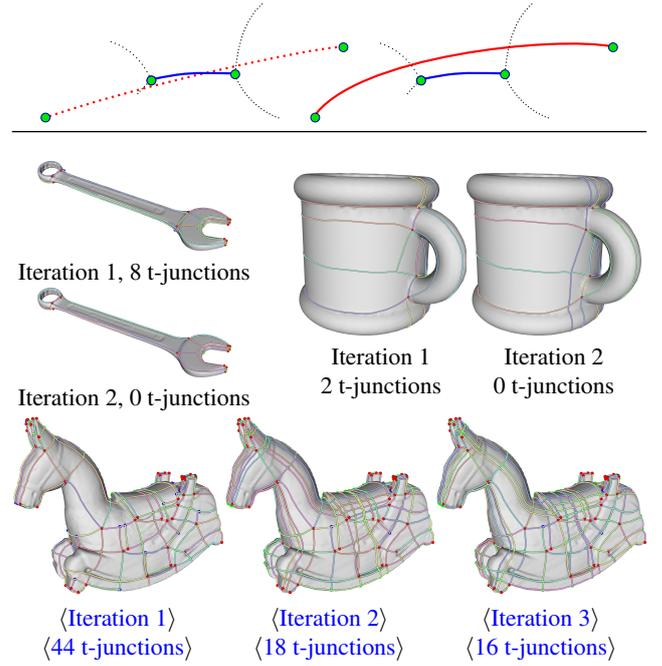
**Figure 7:** *Top:* The dotted red separatrix on the left would be shorter than the continuous red separatrix on the right. However, adding the blue separatrix to the layout in a first run prevents the insertion of the dotted red separatrix, while the continuous red separatrix is found as best shot, compatible with the blue constraint. *Bottom:* a few iterations allow us to remove or considerably reduce the number of t-junctions in the final layout.
