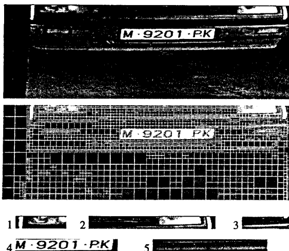
Fig.4 – Sample of the system operation Top: input field – Middle: Structural decomposition Bottom: extracted candidate stripes
