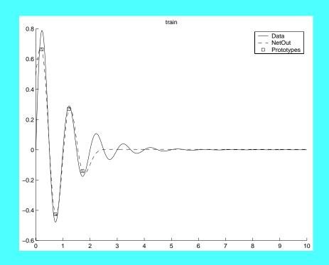
$f_1$  (continuous line) and the output of PRBFN (dashed line), the prototypes are shown as rectangles.
