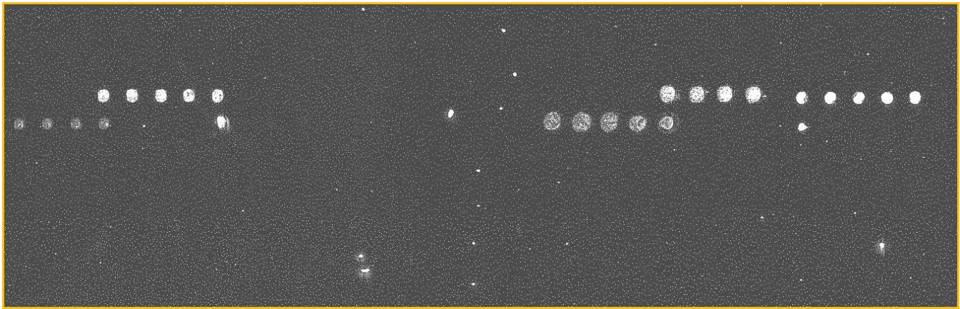
Fig. 1. A sample image produced by the scanner. It is possible to distinguish spots with positive or intermediate activation and outliers, as for instance the bright spots in the bottom area of the image.
